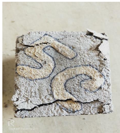
Fig 5: Failure pattern of Mortar cube with 5% sand replaced by crumb rubber
