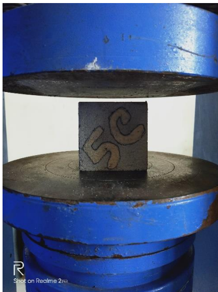
Picture 2: Compression Testing of Mortar Sample with 5% sand replaced with Crumb Rubber
