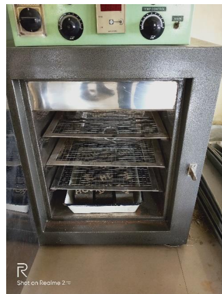
Picture 3: 12 samples of mortar cube inside heater for Heat Test
