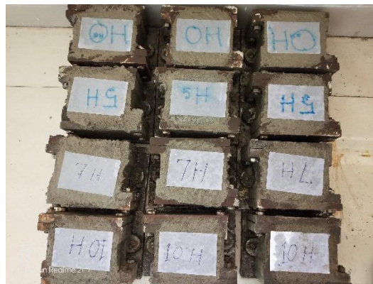
Picture 4: Prepared mortar cube sample for heat test
